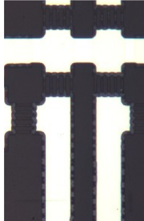
Array with data lines and TFT stack etched away to reveal how undercut has isolated the gate lines
