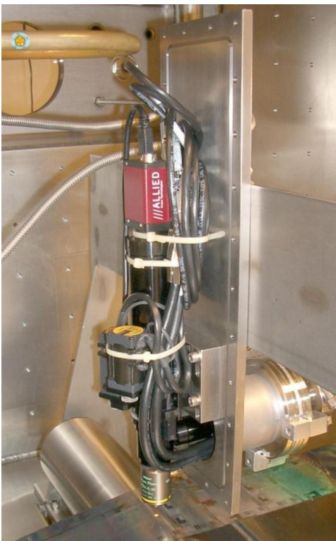
Figure 1 Inspection microscope inside the roll-to-roll RIE system
